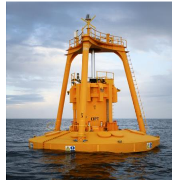
Fig. 2. One popular example of a body PAs that may self-react is the OPT power buoy device [25].
