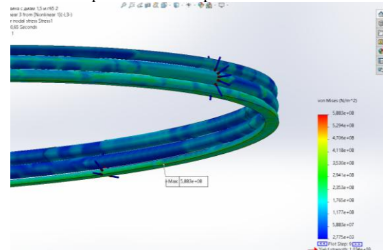
Fig . 8. Results of stress at operating values of compression and temperature of 200 °C
