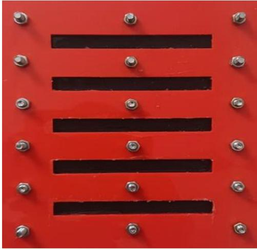
Fig. 9. Fatigue specimens mold
