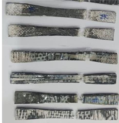
Fig. 5. Tested tensile specimens
