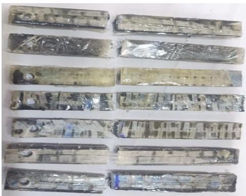
Fig. 11. Tested fatigue specimens
