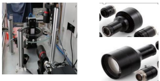
Fig. 6. Image and apparatus of the experimental setup: a) apphire substrate and detection images, b) telecentric imaging lens device and components
