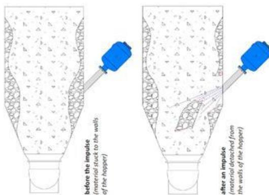
Fig. 1. The idea of using a gas pulser
