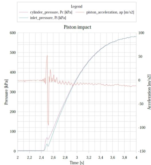
Fig. 16. Characteristics of the acceleration value upon piston impact
