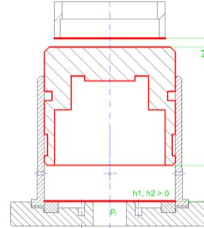
Fig. 14. Piston position during equilibrium experiment
