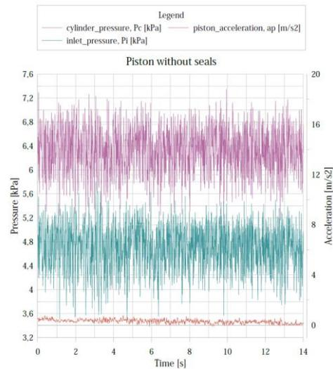
Fig. 15. The piston in equilibrium. Fourth repetition of the experiment
