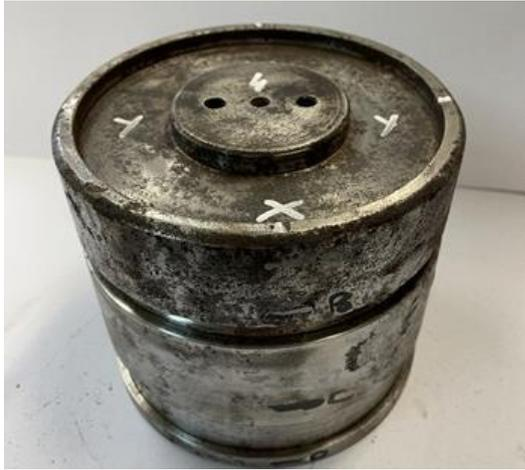
Fig. 6. Piston after 2000 cycles of work.
