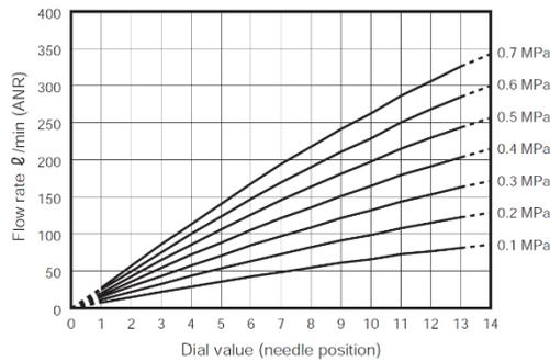
Fig. 11. Flow characteristics of proportional valve depicted earlier in Fig 10a
