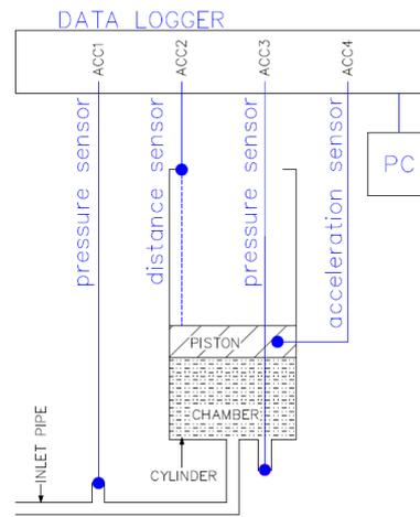
Fig. 12. Diagram of the measurement system
