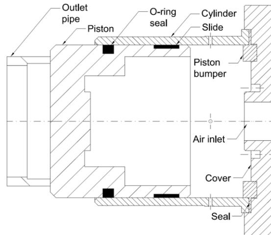
Fig. 9. Cross section of the piston in the cylinder and discharge pipe
