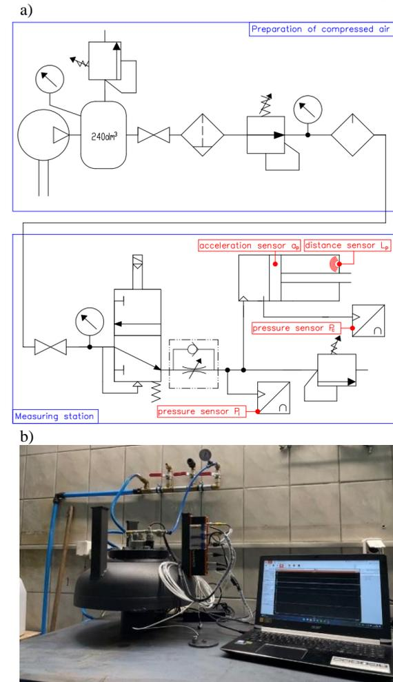
Fig. 10. Diagram of the pneumatic system and the measurement setup (a) and photo of the measurement station (b)
