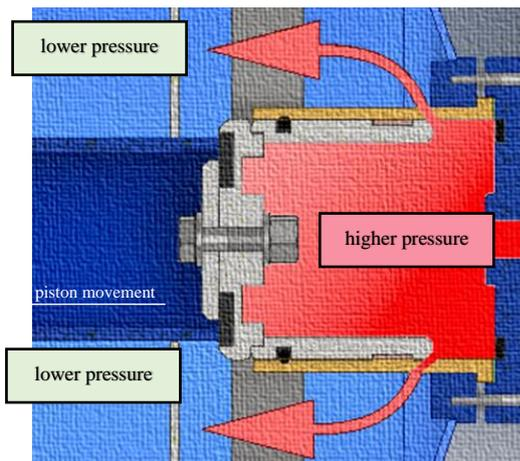
Fig. 3. 1st stable piston position: container charging
