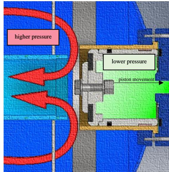
Fig. 4. 2nd stable piston position: container air discharge
