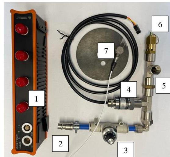
Fig. 13. Components of the measurement system (1 - Data logger, 2 - Air supply, 3 - Throttle valve, 4 - Pressure sensor, 5 - Air supply to the air chamber, 6 - Safety valve, 7 - Accelerometer)
