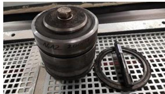
Fig. 5. Damaged front seal
