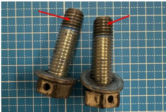
Fig. 7. Damaged threads of the main nut
