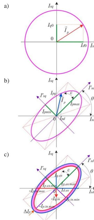
Fig. 3. Figure of the Park's vector: *a* – for an intact machine and a symmetrical system of supply voltages, *b* – with inter-turn shorting of the stator winding and asymmetry of the supply voltages; *c* – in case of defect to the structure of the short-circuited rotor winding and asymmetry of the supply voltages
