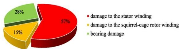
Fig. 1. Distribution of failures according to the main structural elements of an asynchronous machine
