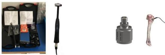
(a) Impulse Hammer (b) Accelerometer type YMC161A
