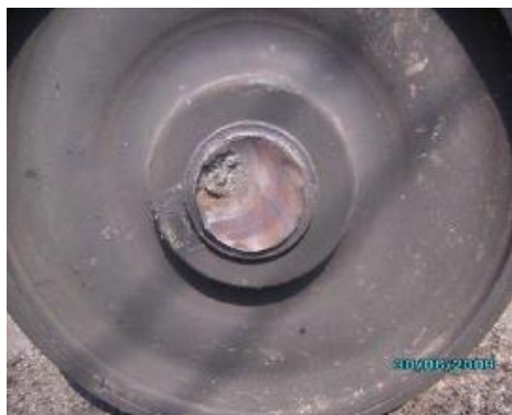
Fig. 8. Axle fillet fracture that caused the accident at Viareggio station, Italy [22]
