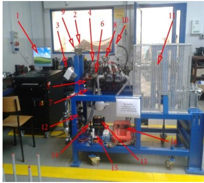
Fig. 4. Components of the measuring stand: 1 – computer, 2 – throttle and choke levers, 3 – desktop, 4 – air filter, 5 – oil tank, 6 – starter, 7 – regulator, 8 – magnetos, 9 – oil pressure gauge, 10 – oil cooler, 11 – water brake, 12 – coolant radiator, 13 – battery, 14 – main power switch, 15 – electromagnet, 16 – fuel tank
