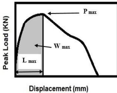
Fig. 1. Load-displacement curve in a tensile test;  $W_{max}$ : energy absorption;  $P_{max}$ : peak load;  $L_{max}$ : elongation at peak load (25)
