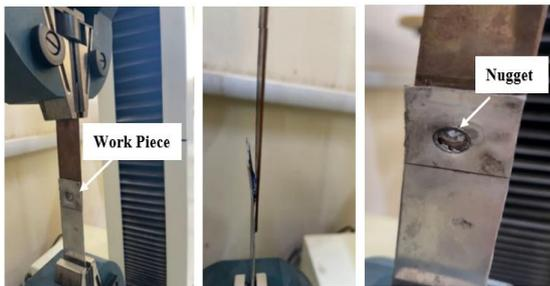
Fig. 13. Tensile test for welded joints
