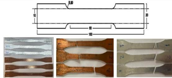
Fig. 4. Tensile-shear specimens and dimensions
