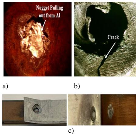
Fig. 15. PF modes in Al-Cu RSW: a) Cu side pull out the Al-nugget side, 10 x; b) Al-nugget side, 10 x; c) Cu and Al nugget after failure
