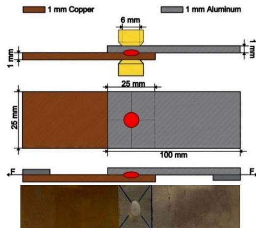
Fig. 5. RSW specimen dimensions
