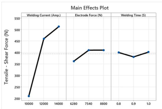
Fig. 3. Main effects plot of tensile force
