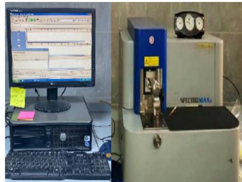
Fig. 2. Optical Emission Spectrometer
