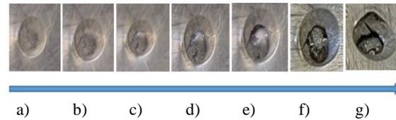
Fig. 14. Initiation with propagation of crack in tensile shear test during consecutive time periods: a) 0 min; b) 1 min; c) 2 min; d) 3 min; e) 4 min; f) 5 min; g) final failure mode
