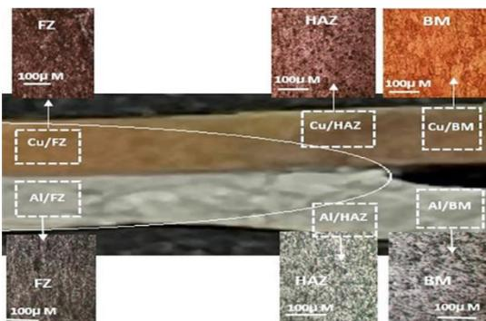
Fig. 19. RSW zones of the Al-Cu Joint
