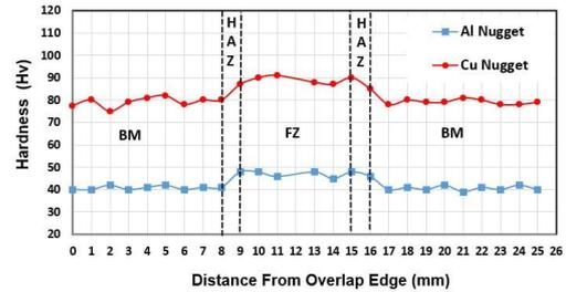
Fig. 17. Surface hardness for RSW joint
