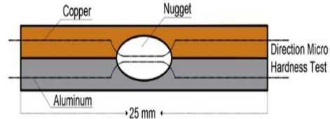
Fig. 9. Cross-section micro hardness
