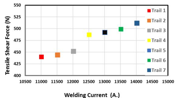
Fig. 12. Effect of welding current on RSW tensile shear force
