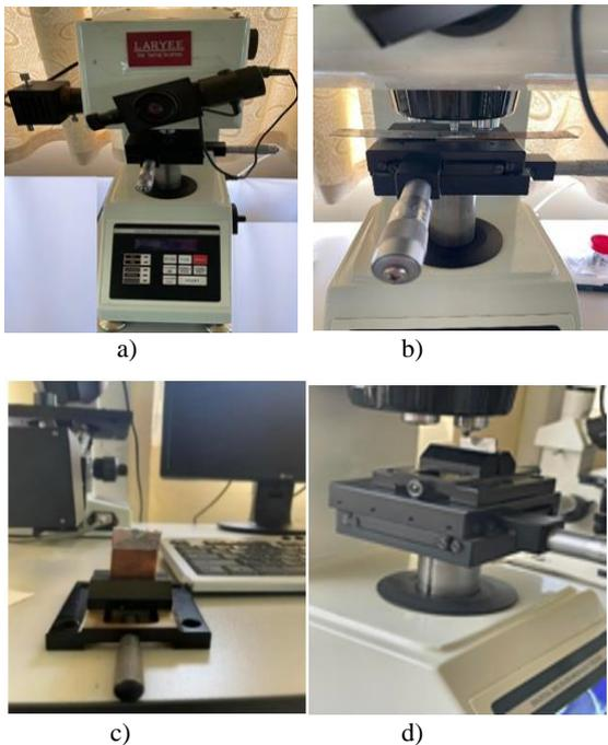
Fig. 8. a) Vickers Micro Hardness Testing device; b) Surface Micro Hardness Measurement for RSW Joint; c) Cross-Section Micro Hardness Specimen with Special Grip; d) Cross-Section Micro hardness measurement
