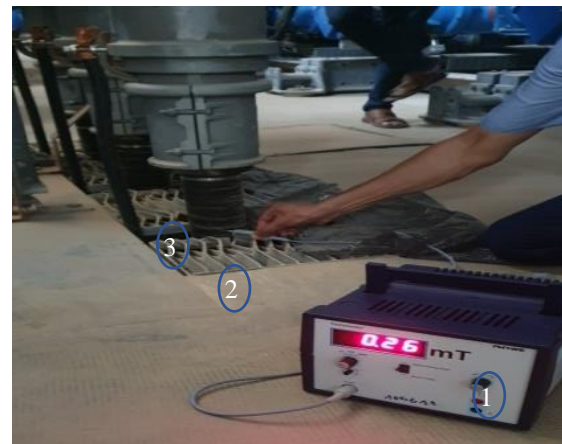
Fig. 4. Experimental setup of magnetic flux density measurement: 1- Teslameter, 2- probe 3-Underground power cable
