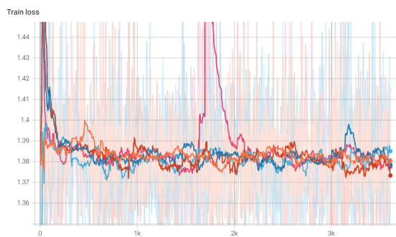
Fig. 4. Training loss of several runs using the full wav2vec transformer. In all tested setups, the transformer model failed to converge.
