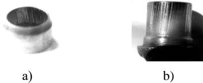
Fig. 4. The appearance of worn parts («false brining») of the bearing assembly of the crosspiece a) – the bearing cage; b) – the axle of the crosspiece
