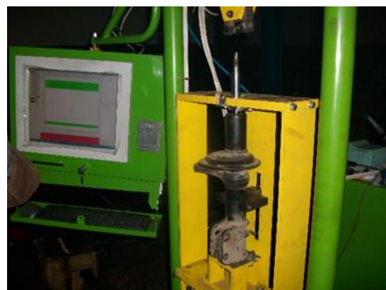
Fig. 9. Diagnostics of the speed characteristics of the front strut of the shock absorber with an innovative repair kit
