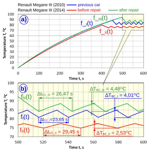
Fig. 15. Comparison of the functions used to model the operation of the cooling system
