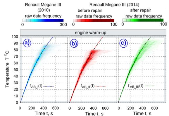
Fig. 12. Functions modelling cold engine warm-up and the frequency of individual data points occurrence
