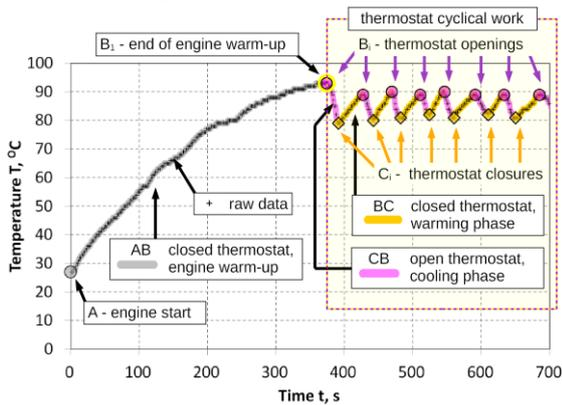
Fig. 10. Example of engine temperature variation during 700 s of operation with characteristic points marked
