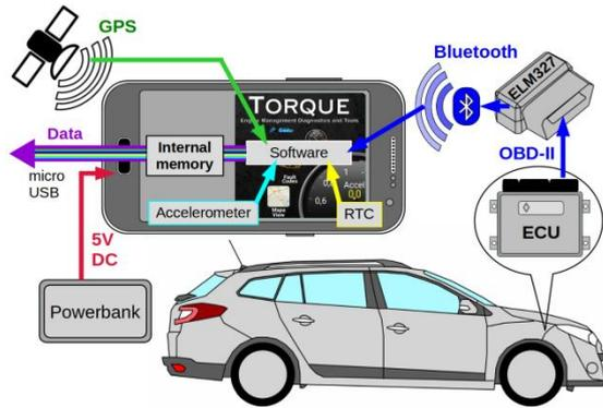
Fig. 5. Scheme of the data acquisition system
