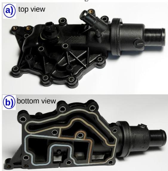
Fig. 4. K4M engine thermostat assembly
