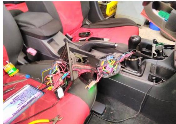
Fig. 4. Installation of a Raspberry Pi.4 computer in a Mitsubishi LANCER
