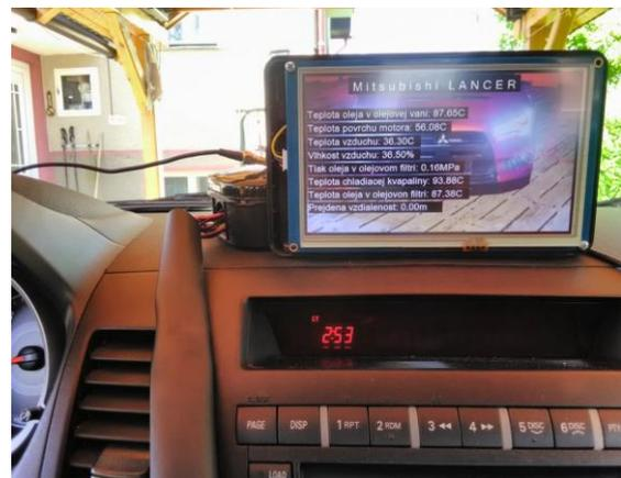
Fig. 5. Installed display unit of measuring station in passenger car Mitsubishi LANCER 1.5
