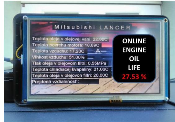
Fig. 7. Display unit with approximate calculation of the current remaining engine oil life
