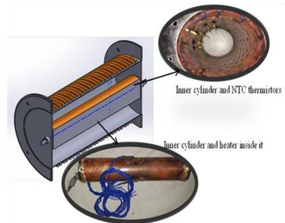
Fig. 1. Specimens used in the experimental tests
