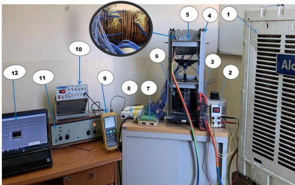
Fig. 4. The experimental test rig. 1: Closed cooling water circuit, 2: Variac, 3: Digital clamp meter, 4: Iron structure, 5: Test section, 6: Vibration exciter, 7: Electric card and its connection wires, 8: National instrument data acquisition, 9: Vibration meter, 10: Function generator, 11: power amplifier, 12: Personal computer (PC)
