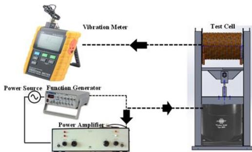
Fig. 2. Test cell with vibration instruments connection scheme
