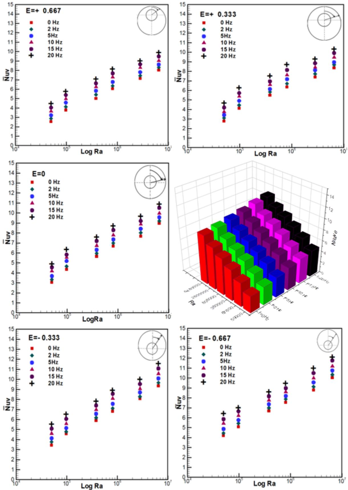
Fig.9. Average Nusselt versus with the logarithmic of Rayleigh number at all applied frequencies for each eccentric
