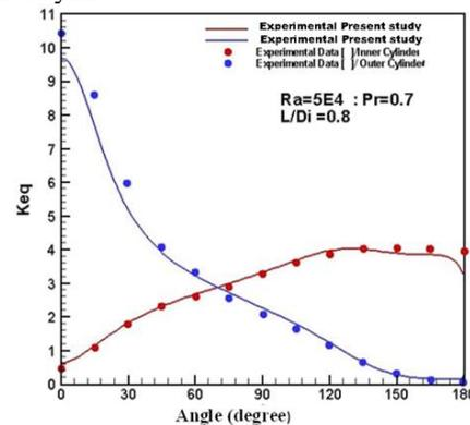
Fig. 5. Comparison of the concentric local heat transfer coefficients at  $\varepsilon = 0$  from [1]
