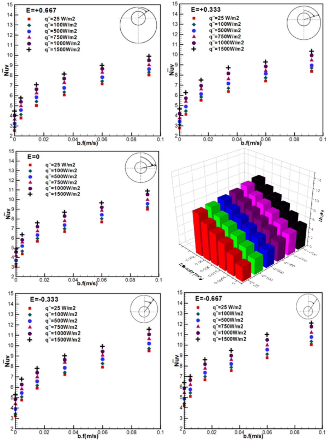
Fig. 7. The effect of vibration intensity on the average Nusselt number for all applied heat flux at each eccentricity.
