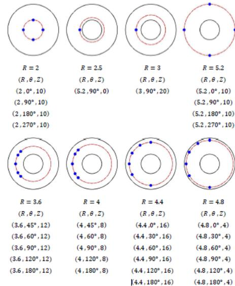
Fig. 3. Schematic representation for NTC thermistors and their fixing on the inner and outer cylinders
