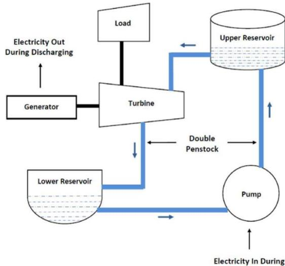
Fig. 4. Pumped hydroelectric storage system (PHES) [49]
