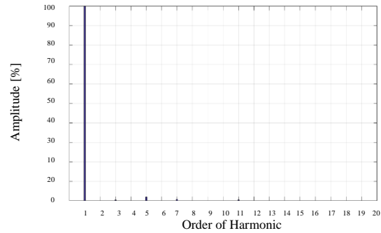
Fig. 7. Harmonic spectrum of Grid current
