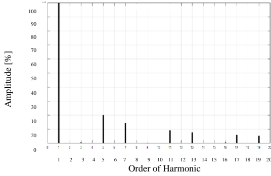
Fig. 10. Harmonic spectrum of load current
