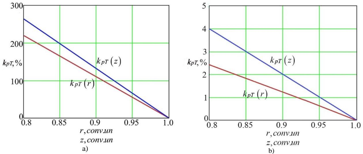
Fig. 2. Graphs of the dependence of the pulsation factor of the electromagnetic torque with a change in the active r and complex z resistance of the phase A of the stator y: a) idle mode; b) nominal mode
