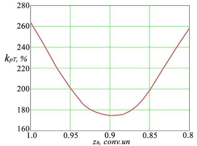
Fig. 3. Graph of the dependence of the pulsation factor of the electromagnetic torque when the complex resistance of phase B changes with a damaged phase A by 20%
