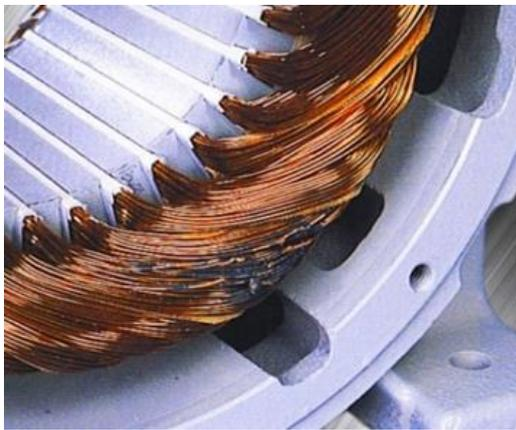
Fig. 1. Turn-to-turn short circuits in the stator winding
