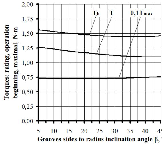
Fig. 5. Influence of grooves sides to radius inclination angle on the clutch load capacity
