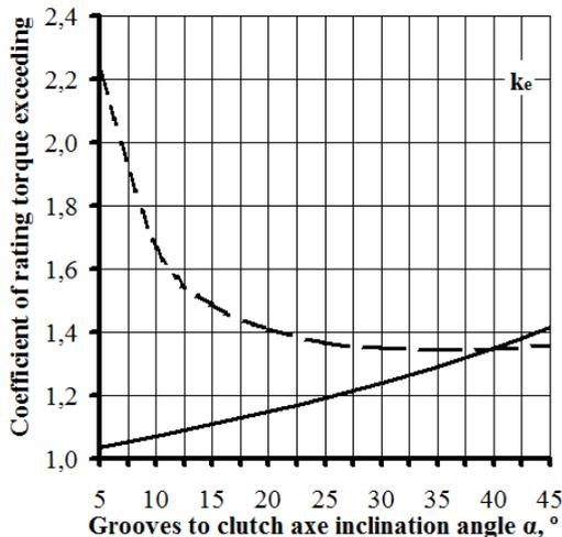
Fig. 8. Influence of the semi-couplings grooves inclination angle on the rating torque exceeding coefficient
