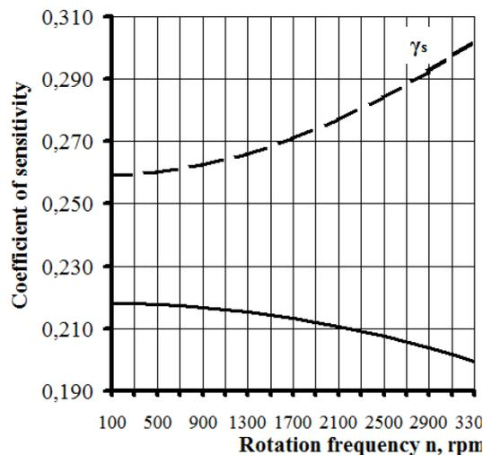
Fig. 13. Influence of the clutch rotating frequency on the sensitivity coefficient
