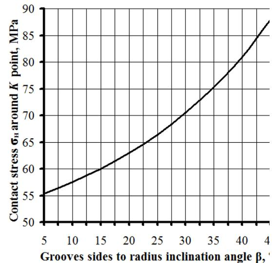
Fig. 6. Influence of grooves sides to radius inclination angle on clutch parts contact stress around K point
