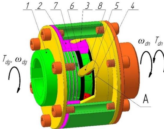
Fig. 1. Safety-overrunning clutch with inclined grooves sides scheme:
