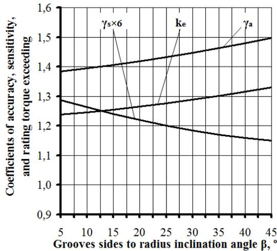
Fig. 7. Influence of grooves sides to radius inclination angle on accuracy, rating torque exceeding, and clutch sensitivity coefficients
