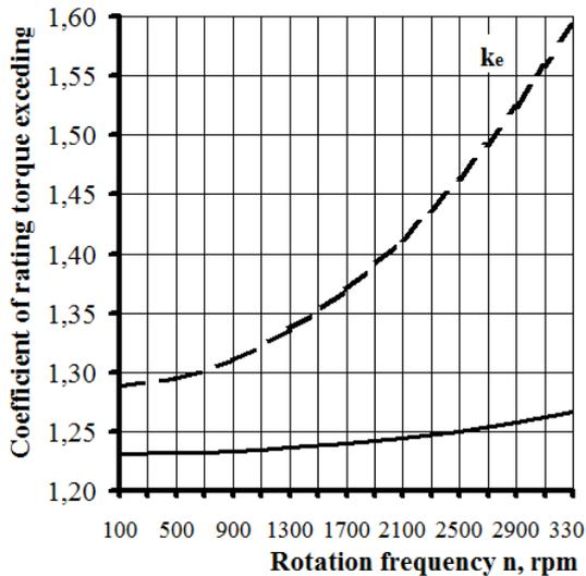
Fig. 11. Influence of the clutch rotating frequency on the rating torque exceeding coefficient
