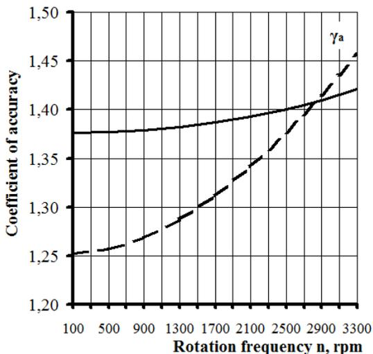
Fig. 12. Influence of the clutch rotating frequency on the accuracy coefficient
