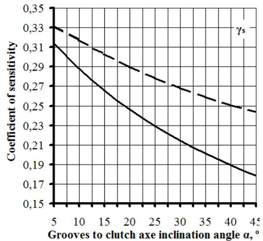
Fig. 10. Influence of the half-couplings grooves inclination angle on the sensitivity coefficient
