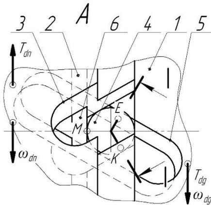
Fig. 2. Inclined grooves sides scheme (view A by fig. 1)
