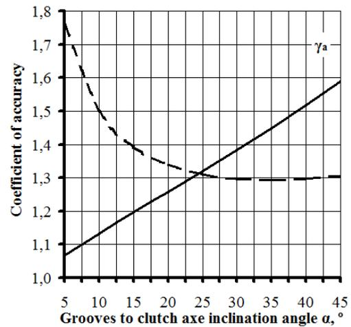
Fig. 9. Influence of the semi-couplings grooves inclination angle on the accuracy coefficient
