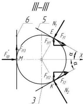
Fig. 4. Ball force diagram at the clutch overload mode beginning
