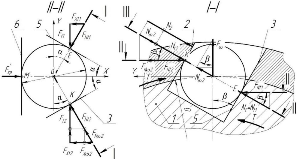
Fig. 3. Clutch parts force interaction diagram
