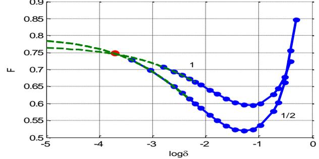
Fig. 5. The relative maximum stress in a plate made of material EF; 1 - circular holes, 1/2 - elliptical holes
