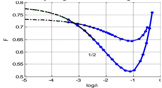
Fig. 2. The relative maximum stress in isotropic plate, 1 - circular holes, 1/2 - elliptical holes
