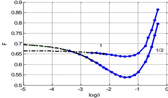
Fig. 4. The relative maximum stress in a plate made of material CF1<sub>90</sub>; 1 - circular holes, 1/2 - elliptical holes
