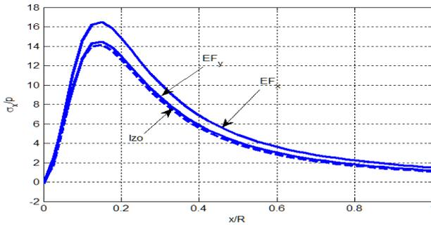
Fig. 10. Stress at the boundary of the half-plane (EF material end isotropic material)
