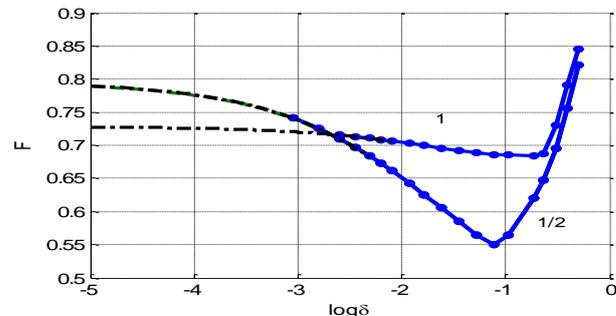
Fig. 7. The relative maximum stress in a plate made of material EF<sub>45</sub>. 1 - circular holes, 1/2 - elliptical holes
