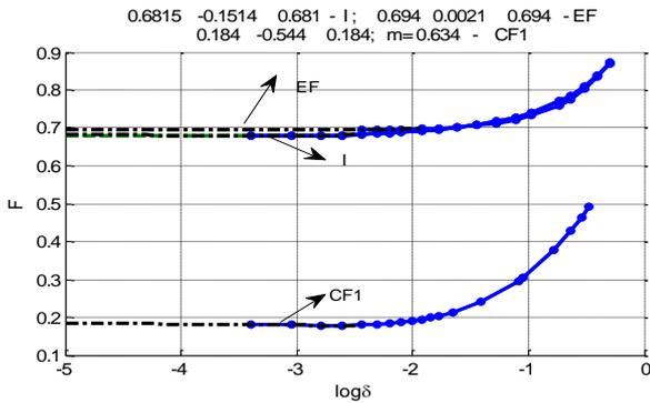
Fig. 8. The relative maximum stress in a plate with elongated ellipse holes at  $b/a=2$
