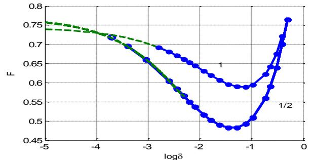
Fig. 6. The relative maximum stress in a plate made of material EF<sub>90</sub>; 1 - circular holes, 1/2 - elliptical holes
