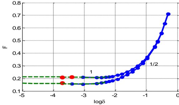
Fig. 3. The relative maximum stress in a plate made of material CF1, 1 - circular holes, 1/2 - elliptical holes
