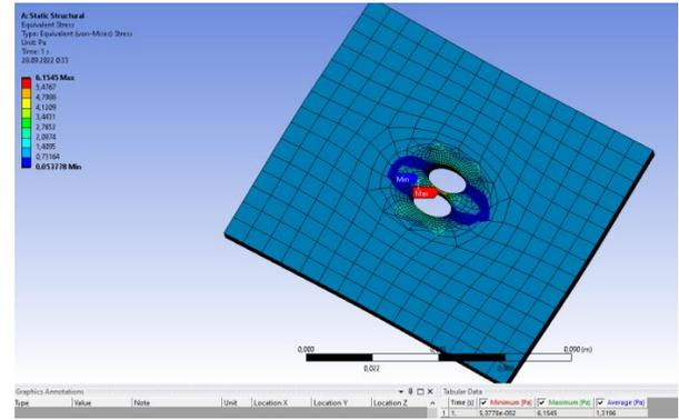
Fig. 10. Relative maximum stresses in the plane with a two circular hole (isotropic material)
