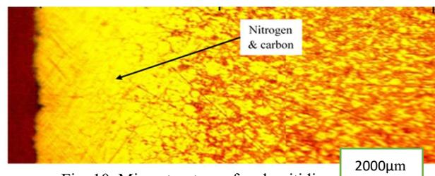
Fig. 10. Microstructure of carbonitriding material
