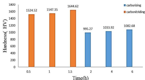
Fig. 11. Influence holding (soaking) time of carbonitriding and carburizing on hardness of low carbon steel specimens
