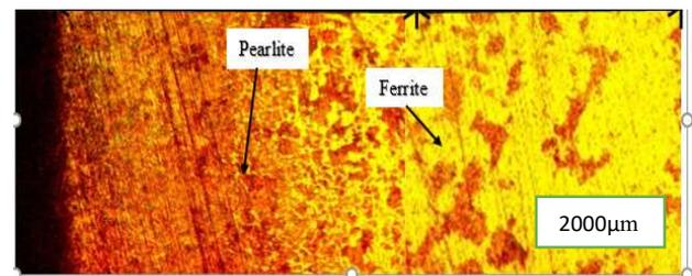
Fig. 9. Microstructure of carburized material
