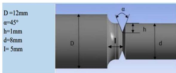
Fig. 4. Dimensions of V shape notch specimens
