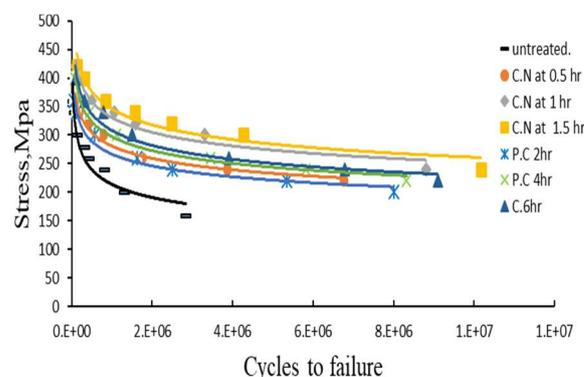
Fig. 14. Comparison between effect surface hardening (pack carburizing, carbonitriding) on S-N curve of fatigue test specimens at varying time with un-treated
