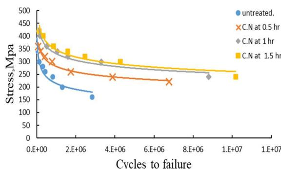
Fig. 13. Effect surface hardening (carbonitriding) on S-N curve of fatigue test specimens at varying time with un-treated
