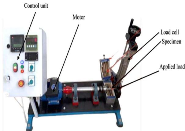
Fig. 7. Fatigue testing machine
