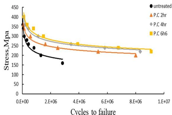
Fig. 12. Effect surface hardening (pack carburizing) on S-N curve of fatigue test specimens at varying time with un-treated
