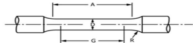
Fig. 1. Schematic of tensile test specimen according to the specification of (ASTM-A 370)
