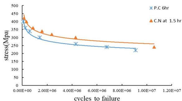
Fig. 15. Comparison S-N curve (carbonitriding at time 1.5h and pack carburizing at time 6h)
