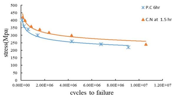
Fig. 15. Comparison S-N curve (carbonitrid at time 1.5h and pack carburizing at time 6h)
