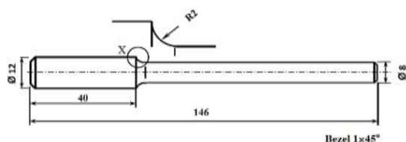
Fig. 3. Schematic diagram for fatigue test specimens
