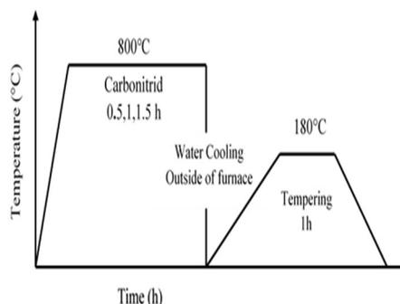
Fig. 6. Heat treatments (cyaniding) for low carbon steel
