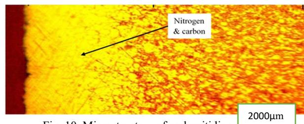
Fig. 10. Microstructure of carbonitriding material
