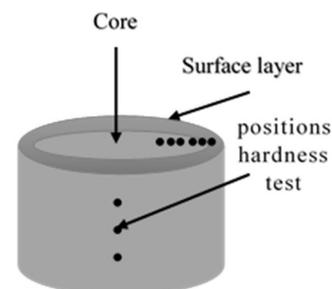
Fig. 2. Schematic for hardness sample
