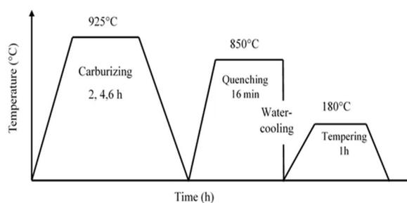
Fig. 5. Heat treatment (pack carburizing)
