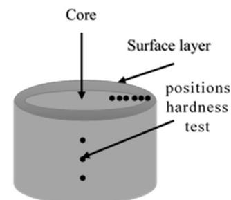
Fig. 2. Schematic for hardness sample
