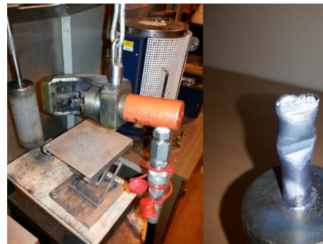
Fig. 6. Seal the capsule using a hydraulic press
