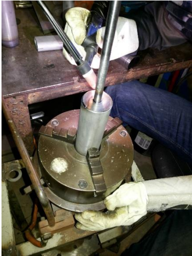
Fig. 3. Welding HIP mild steel capsule
