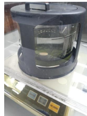
Fig. 11. Density measuring device according to Archimedes principle
