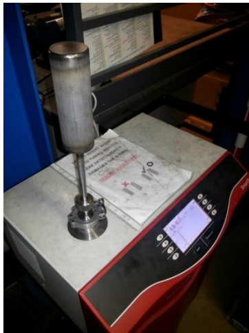
Fig. 4. Inspect the welded capsule to ensure that no gases leak from or into it
