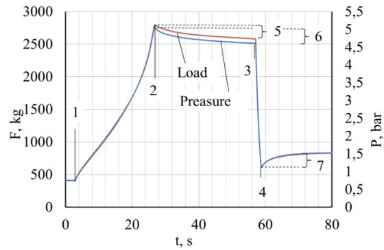
Fig. 5. The oscillogram of the working process of a pneumatic spring with an illustration of the influence of compressed air temperature
