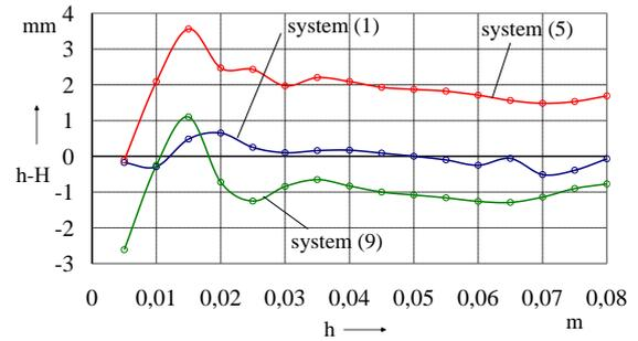
Fig. 13. Comparison of the accuracy of setting the level of the motor vehicle body by the considered regulators
