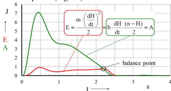
Fig. 10. Illustration of the principle of balancing the operation of the pneumatic spring and the kinetic energy of the vehicle body
