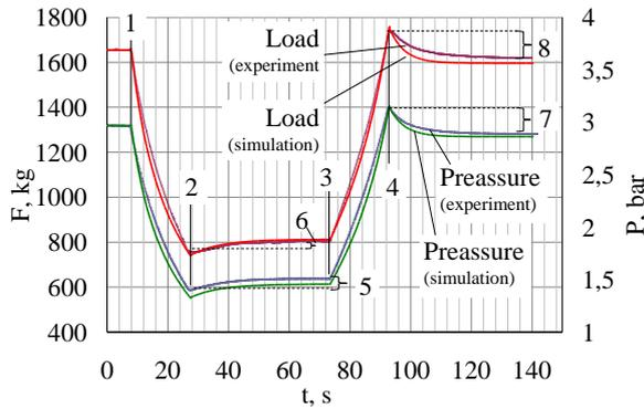
Fig. 6. Verification of the pneumatic spring model
