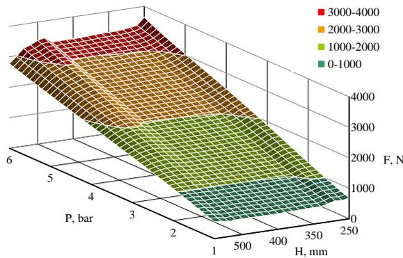
Fig. 3. The load surface of the pneumatic spring
