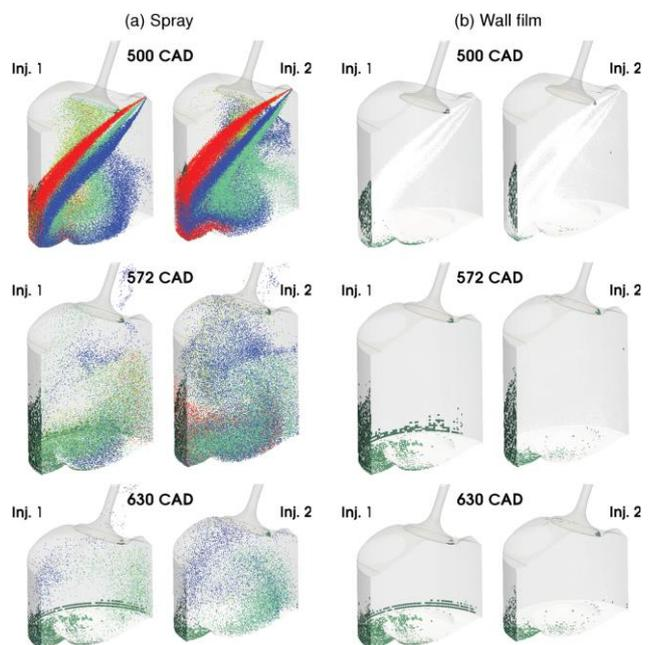
Fig. 9. Computed fuel spray and evolution of liquid film at different times after start of injection and initial point 1, 1500 r / min.: (a) distribution of fuel spray to distinguish the nozzle where each parcel is used so different colour, and (b) assessment of the formation of liquid film. Dark green indicates a liquid-coloured film [23]
