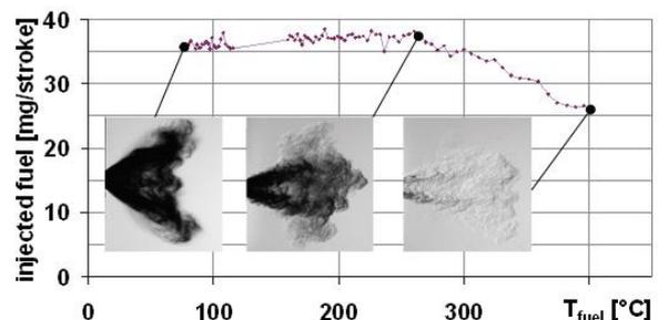
Fig. 10. Impact of high temperature on the flow rate of the fuel mass;  $T_{ch} = 25$  °C,  $P_{ch} = 1$  bar and  $P_{fuel} = 85$  bar, octane fuel No.95 [24]
