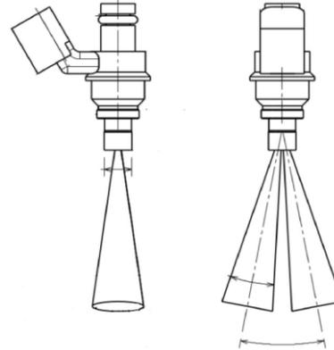
Fig. 3. Views of the fuel injector mounted on the engine (front and lateral). The spray cone's internal and external angles are differentiated by [4]
