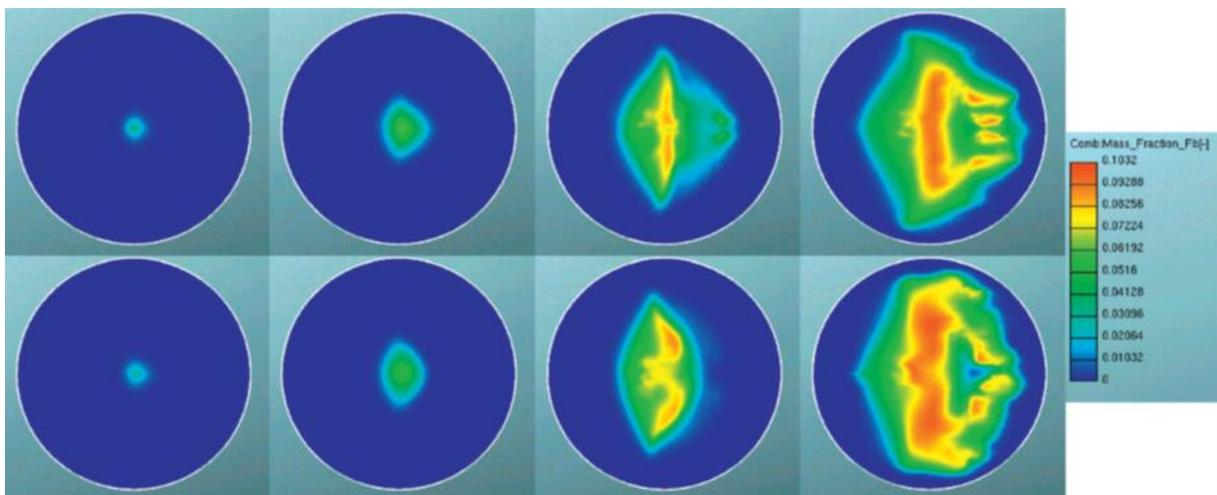
Fig. 7. In the optimum single injection case (top) and double injection case (bottom) at four Crank angles on a plane going through its maximum value, burnt fuel mass fraction [12]
