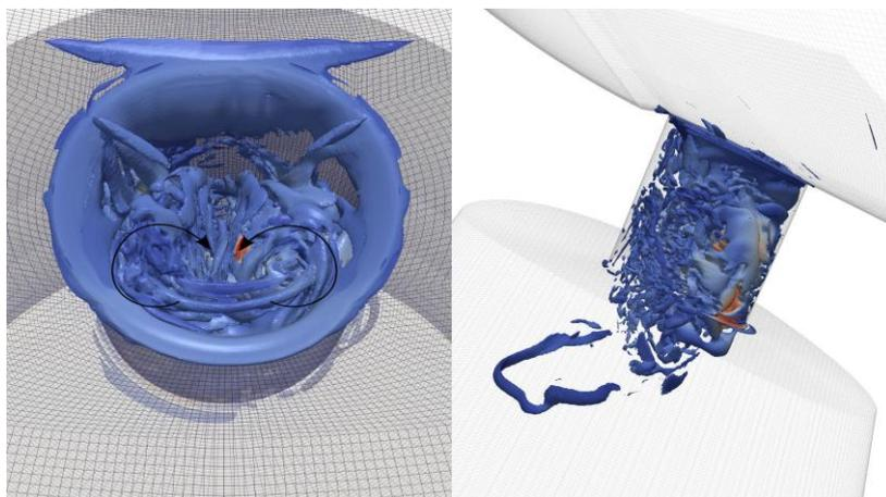
Fig. 4. Structure of the vortical inner nozzle on the left, the upper view, and on the right, the side view from at time  $9.5 \times 10^{-6}$  s, [5]
