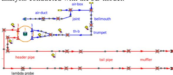
Fig. 2. 1D schematic of the engine GP30 under analysis by [4]
