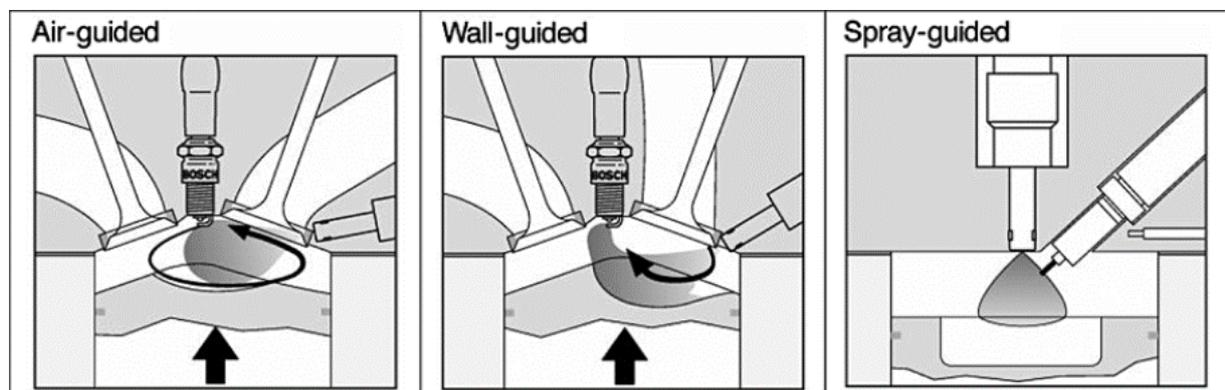
Fig. 8. DISI Combustion systems classifications Preussner et al. [15]
