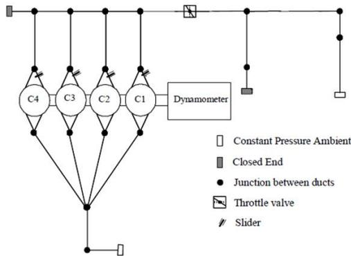
Fig. 1. 1D scheme of the VVT type engine [3]
