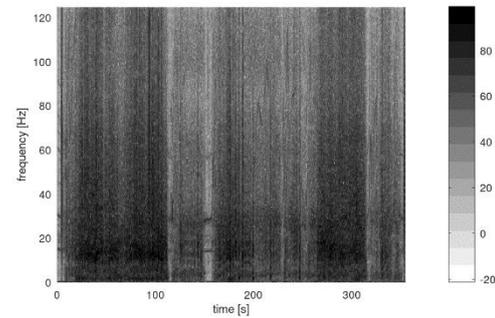
Fig. 5. Spectrogram of Z-axis acceleration waveform obtained from ADIS16470AMLZ
