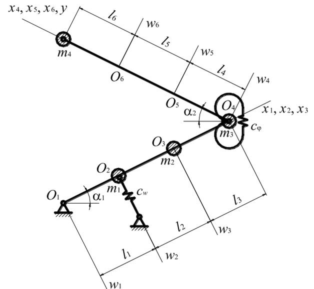
Fig. 1. Calculation scheme of a two-link mechanical system of a robot manipulator
