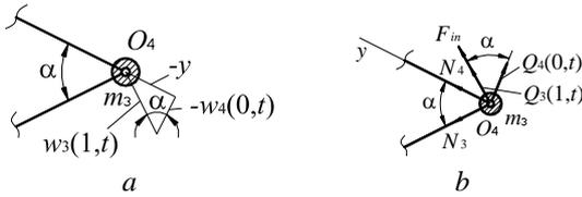
Fig. 2. Diagram of (a) the displacements of the hinge by which the robot links are joined and (b) the forces acting on the hinge
