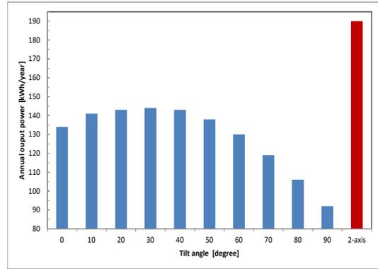
Fig. 11 Annual AC power production for different tilt angles and two-axis tracking considering cell temperature-related losses at Najaf city, Iraq.
