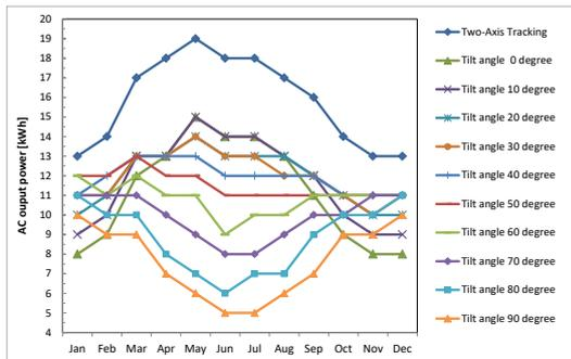
Fig. 10 Monthly AC power production for different tilt angles and two-axis tracking considering cell temperature-related losses at Najaf city, Iraq
