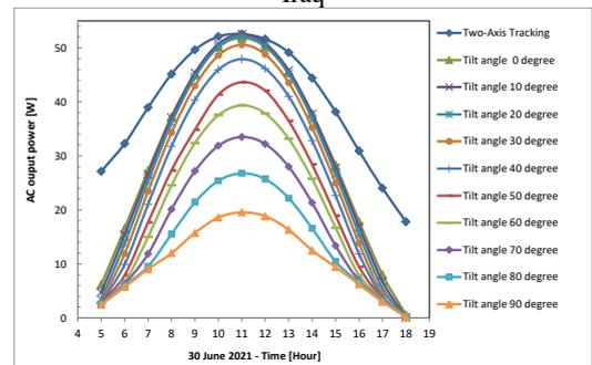
Fig. 14 Hourly AC power production for different tilt angles and two-axis tracking considering cell temperature-related losses at Najaf city, Iraq.
