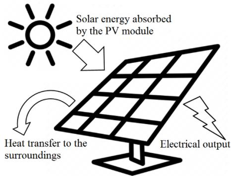
Fig. 4 The energy balance for the PV module.
