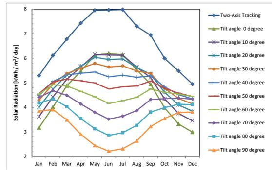
Fig. 5. Daily solar radiation for different tilt angles and two-axis tracking at Najaf city, Iraq.
