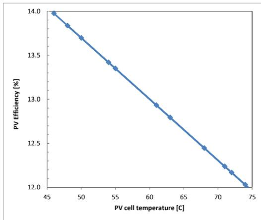
Fig. 9. The changes in the PV efficiency with PV cell temperature.
