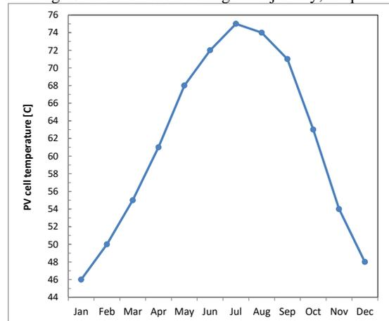
Fig. 6. Monthly average PV cell temperature.
