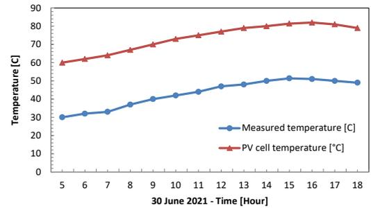
Fig. 12. The measured temperature at approximately two meters above the surface of an open field and the estimated PV cell temperature for a summer day of 30 June 2021.
