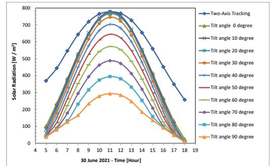
Figure 13 Hourly solar radiation for different tilt angles and two-axis tracking at Najaf city, Iraq
