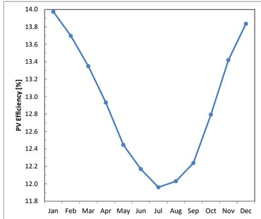
Fig. 8. Monthly average PV efficiency.
