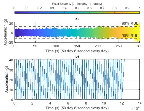
Fig. 2. Signals in the dataset, over 50 days with 6 second per day, a) cumulative vibration and b) tachometer
