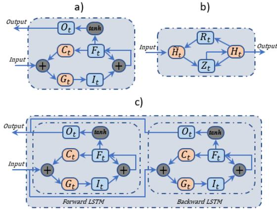
Fig. 4. Main recurrent cells internal structures, a) LSTM, b) GRU and c) BiLSTM
