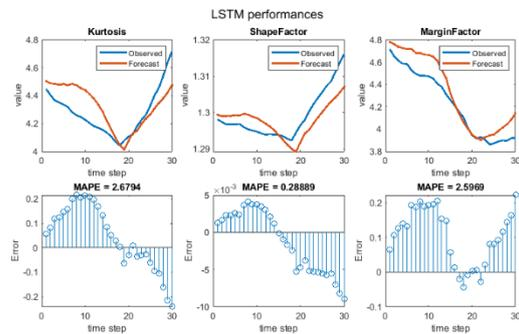
Fig. 11. Values predicted by LSTM, as well as testing data and the related MAPE
