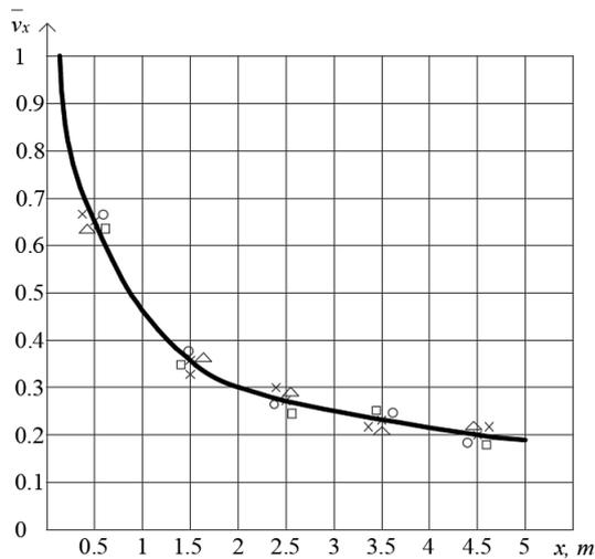
Fig. 4. Graph of the dependence of the relative axial velocity of a plane jet on the current coordinate
