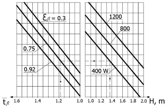
Fig. 2. Dependence of the relative temperature of the irradiation surface on the thermal power of the heater  $Q_{ih}$ , W, height of its installation  $H$ , m and emissivity coefficient of the surface  $\varepsilon_{fl}$
