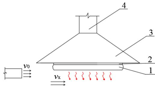
Fig. 6. Scheme of decking of a ventilating air jet on a flat surface at the forced longitudinal flow around an infrared heater of NL - 12R: 1 – infrared emitter; 2 - reflector; 3 - exhaust outlet; 4 - exhaust pipe
