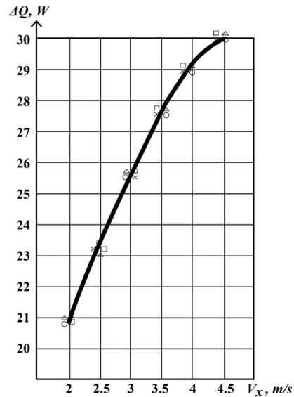
Fig. 7. Graph of the dependence of the amount of saved heat  $\Delta Q$  on the velocity of the flat decking air flow  $v_x$
