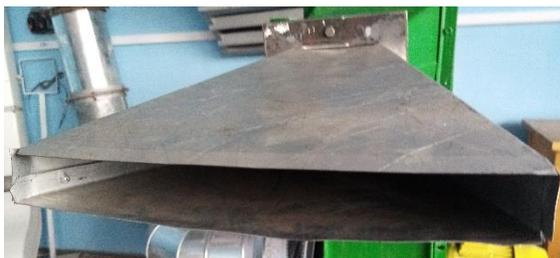
Fig. 3. Experimental installation and nozzle with the aspect ratio  $l/b = 10$  (30x3 cm), which forms a flat compressed air jet
