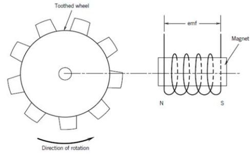
Fig. 5. Angular velocity measurement using a gear wheel and a magnetic pickup [8]
