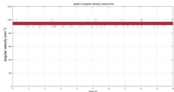
Fig. 11. Angular velocity as a function of time for a constant speed of  $942 \text{ min}^{-1}$
