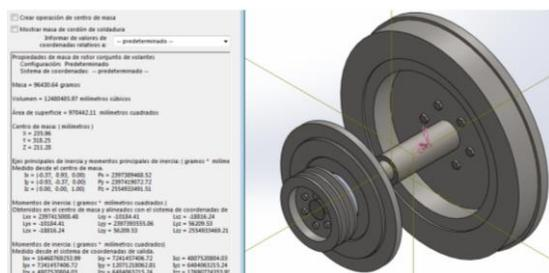
Fig. 15. Determination of the inertial value using the solidworks computational tool
