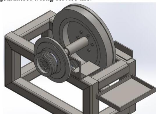
Fig. 3. Shaft assembly with flywheels made in Solidworks
