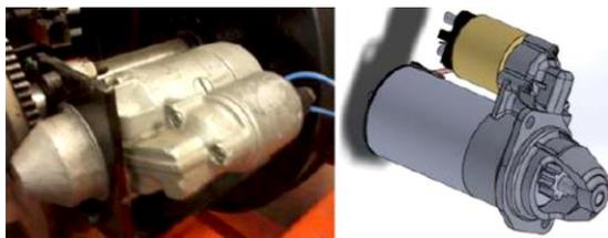
Fig. 1. Starter motor of the test bench with its representation in solidworks
