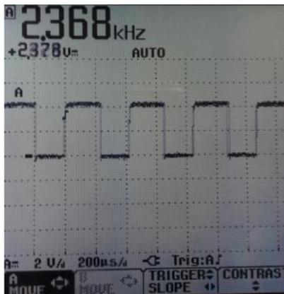
Fig. 8. Electrical voltage signal delivered by the inductive sensor in the oscilloscope
