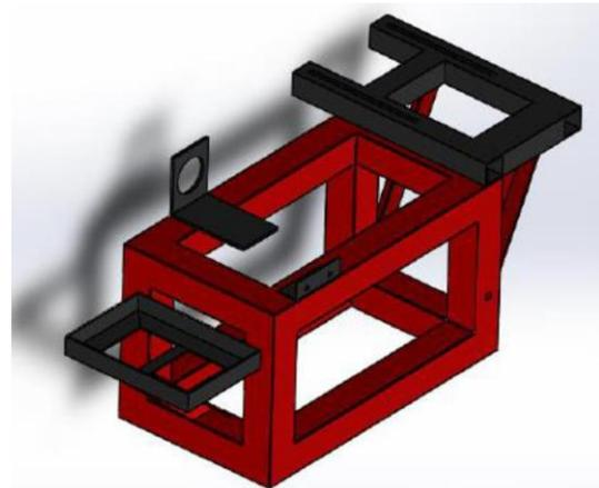
Fig. 2. 3D solid modeling of the metal structure made in Solidworks®
