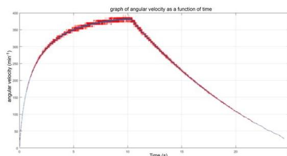
Fig. 17. Angular velocity curve over time during energy accumulation and delivery
