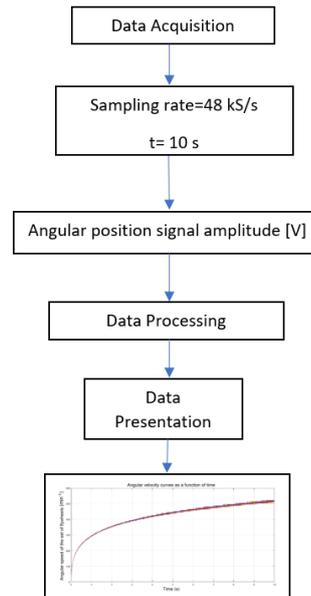
Fig. 9. Flowchart for the algorithm used with the angular position signal
