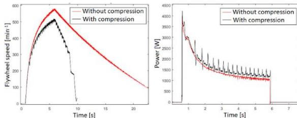
Fig. 18. Flywheel speed during run-up and run-out, and starter power consumed during the motor engine cranking
