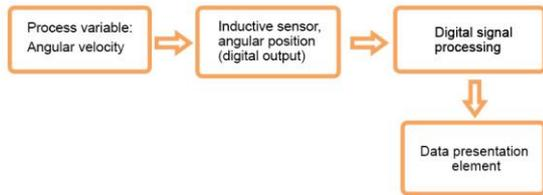
Fig. 7. Block diagram of the angular velocity measurement system.
