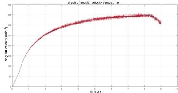
Fig. 13. Angular velocity versus time curve during system startup.
