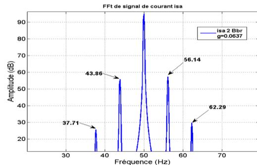
Fig. 10. Current spectrum of phase a, Case of two broken bars
