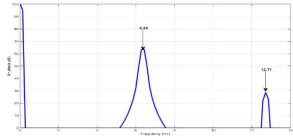
Fig. 16. Park envelope FFT for 1 broken bar
