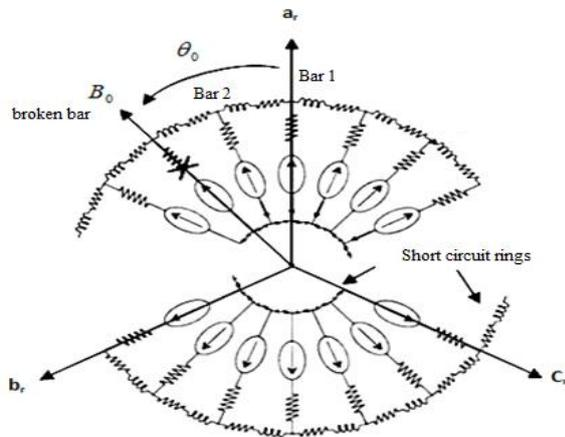
Fig. 3. Model by elementary dipoles of the faulty rotor
