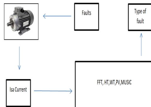
Fig. 1. Schematic representation to detect a rupture of the rotor bars using signal processing
