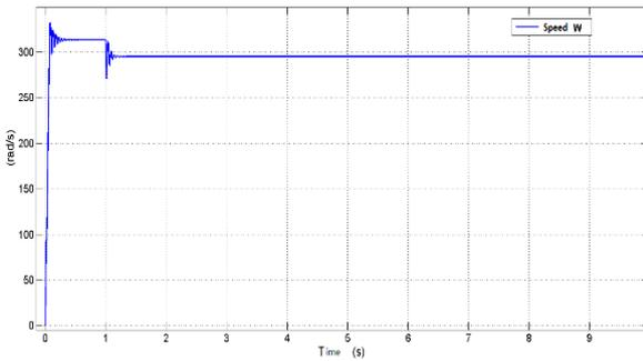
Fig. 5. Rotational speed W simulation of machine in a healthy state
