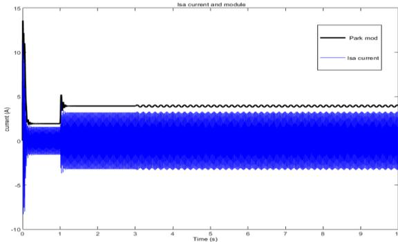
Fig. 13. The modulus of Park's vector approach and stator currents
