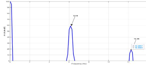
Fig. 17. Park envelope FFT for 2 broken bars
