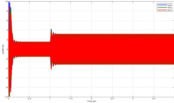
Fig. 4. Courant ISa of machine in a healthy state
