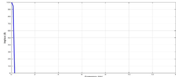
Fig. 15. Park envelope FFT for 0 broken bars
