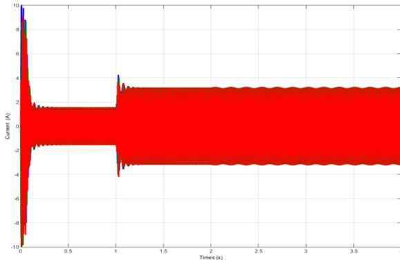
Fig. 6. Courant ISa of machine Case of one broken bars
