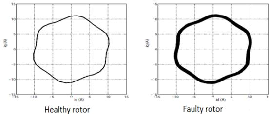
Fig. 12. Park's vector approach of the stator currents
