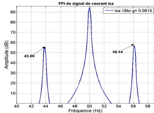
Fig. 9. Current spectrum of phase a, Case of a broken bar
