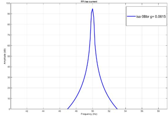
Fig. 8. Current spectrum of phase a, Healthy machine case
