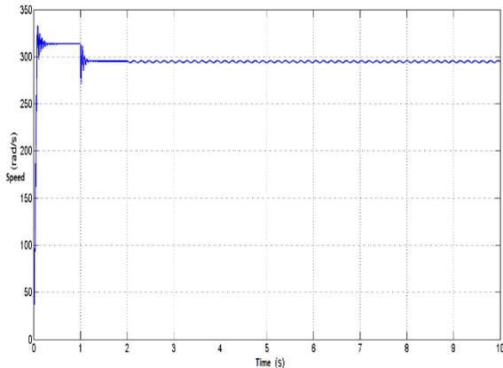
Fig. 7. Rotational speed W of machine Case of one broken bars
