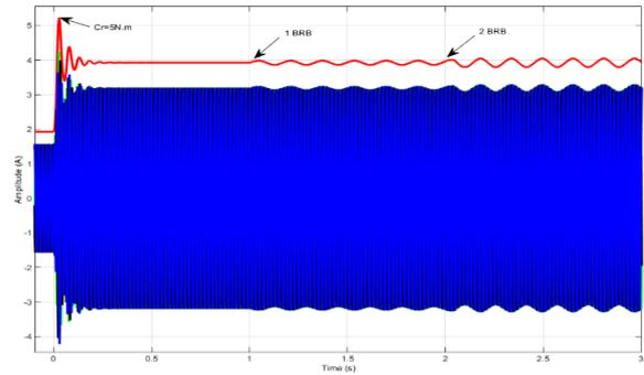
Fig. 14. Zoom of the modulus of the Park vector approach and the stator currents
