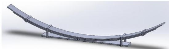
Fig. 15. Leaf spring model resulting from optimization
