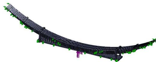
Fig. 10. Finite element model, loading and support fixing of the contact problem
