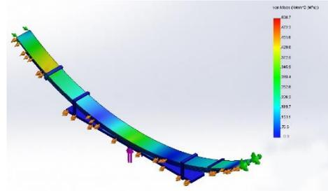
Fig. 17. Equivalent stresses in the contact problem
