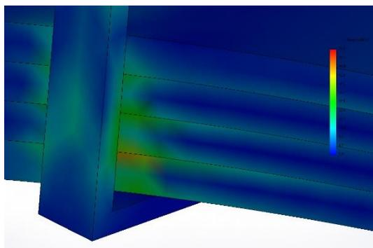
Fig. 13. Contact stresses in the spring leaves
