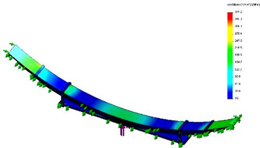
Fig. 11. Equivalent stresses in the contact problem
