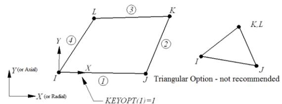
Fig. 3. Geometry of the PLANE 42 element
