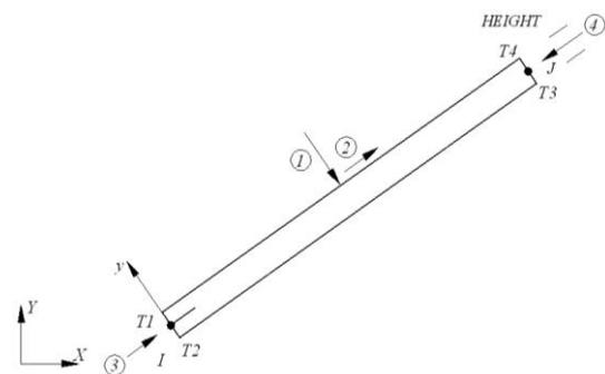
Fig. 4. BEAM3 flat element
