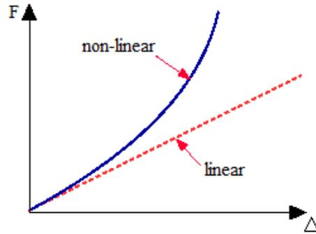
Fig. 9. Linear and nonlinear static analysis dependencies
