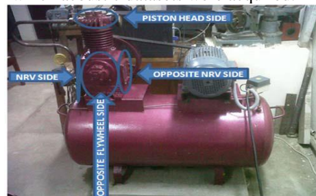
Fig. 1. The air compressor from which acoustic datasets were acquired [12]
