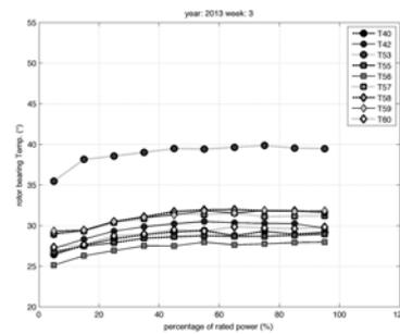
Figure 4. Mean Rotor Bearing Temperature for weekly test period: week 3 of 2013.
