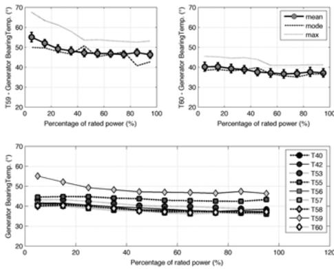
Figure 8. Mean, mode and minimum of Generator Bearing Temperature for turbine T59 (a), T60 (b). Mean of Rotor Bearing Temperature for all the turbines (c). Sample spring period in 2014.
