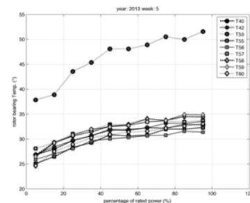
Figure 5. Mean Rotor Bearing Temperature for weekly test period: week 5 of 2013.
