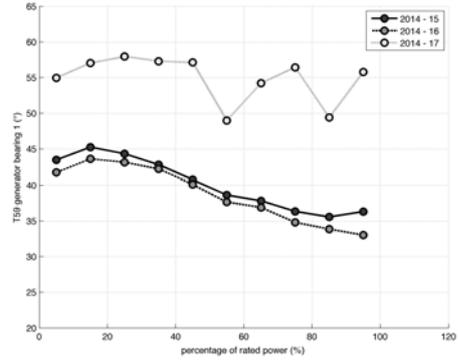
Figure 9. Mean of Generator Bearing Temperature for turbine T59. Sample weekly periods immediately before Figure 6.
