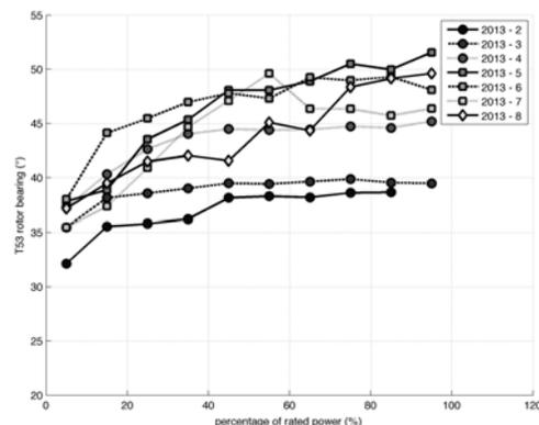
Figure 6. Mean Rotor Bearing Temperature for weekly test periods of turbine T53
