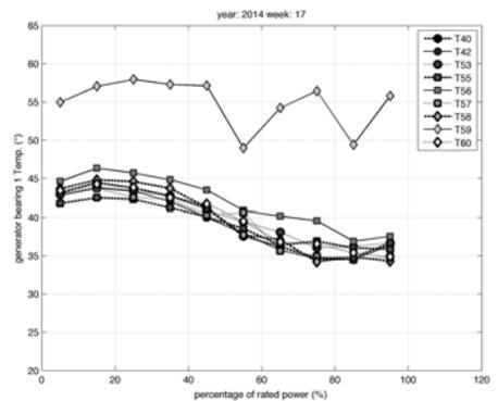
Figure 10. Mean Generator Bearing Temperature for weekly test period: week 17 of 2014.
