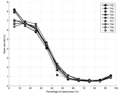
Figure 14. Mean percentage of rotor revolutions per minute standard deviation. Sample period in Spring 2013.
