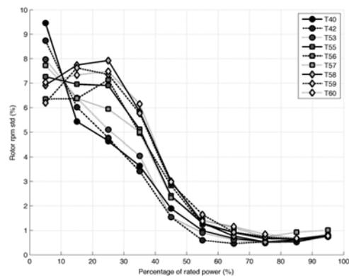
Figure 15. Mean percentage of rotor revolutions per minute standard deviation: 270° sector. Sample period in Spring 2013.
