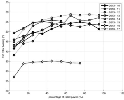
Figure 7. Mean Rotor Bearing Temperature for weekly test periods of turbine T53
