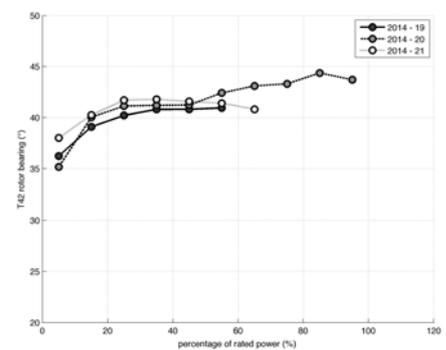
Figure 13. Mean of Rotor Bearing Temperature for turbine T42. Sample weekly periods during Spring 2014.
