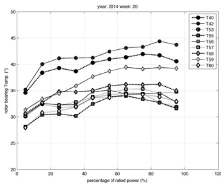
Figure 12. Mean Rotor Bearing Temperature for weekly test period: week 20 of 2014.
