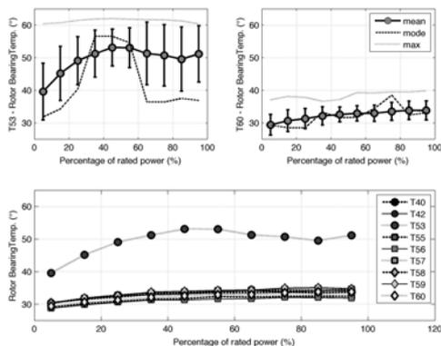
Figure 3: Mean, mode and minimum of Rotor Bearing Temperature for turbine T53 (a), T60 (b). Mean of Rotor Bearing Temperature for all the turbines (c). Sample spring period in 2013.
