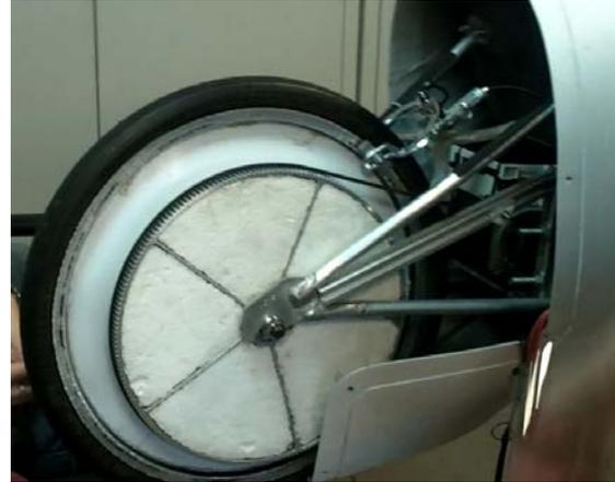
Figure 2 High-speed BLDC motor Dunkermotoren BG75x50 drive system
