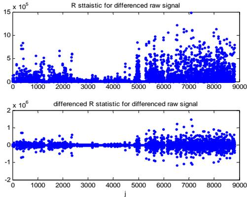
Fig. 9. R and differenced R statistic estimated for differenced raw real signal from Fig. 9 (note that R was estimated with  $k=2$ )
