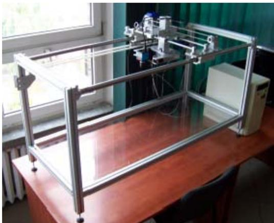
Figure 7. Experimental setup for testing vision systems [25]
