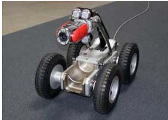
Figure 6. The IPEK vision camera with anti-explosion system [24]
