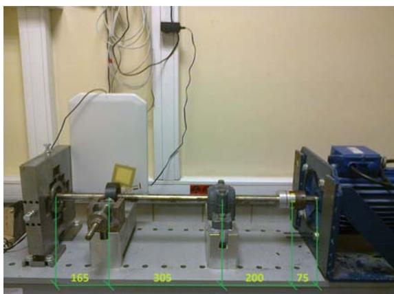
Fig. 2. Laboratory test-stand with the sensing system installed
